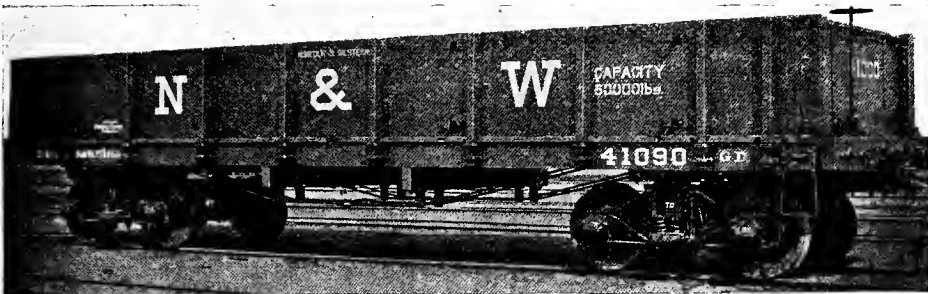
Fig. 23. GONDOLA CAR, WITH DROP-BOTTOM AND DROP-ENDS, FOR COAL, ORE AND LUMBER NORFOLK & WESTERN RAILROAD. Length, 36 ft. 1 in. Capacity, 60,000 lbs. Weight, 27,400 lbs. (Details are shown in Figs. 302-304.)
